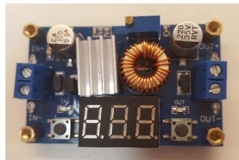
Fig. 28: XL4015 LM2596 Buck Converter
