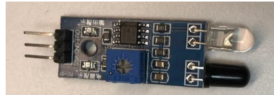
Fig. 10: FC-51 Infrared Sensor
