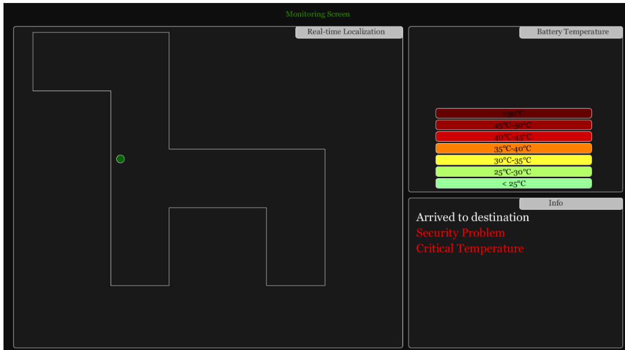
Fig. 42: Complete AGV Monitoring Screen
