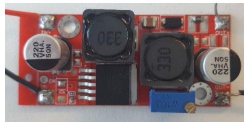
Fig. 31: XL6009 Boost Converter
