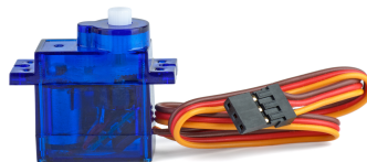
Figure 3.14: 14g Servo Motor with Metallic Gears
