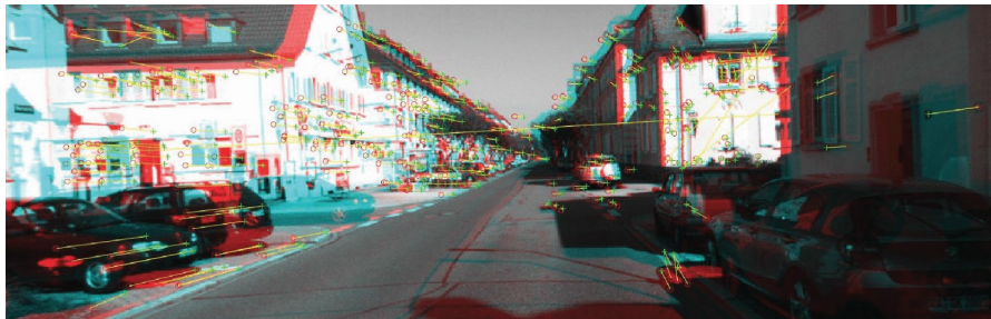
Figure 2.5: An example of SURF feature points matching (Copyright © 2019, IEEE)
